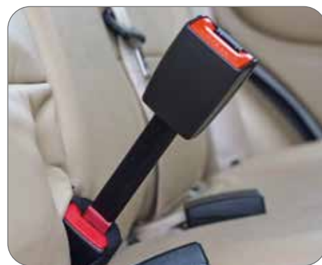
A seatbelt extender can be used to make it easier to buckle the seatbelt
